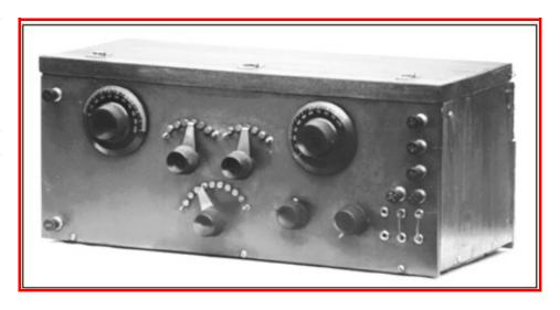
Pictured the improved version of the Reinartz receiver shown in March 1922 QST Magazine. Thanks to Wayne Thalls KB6KN for his input for this article. W8SU 2005
